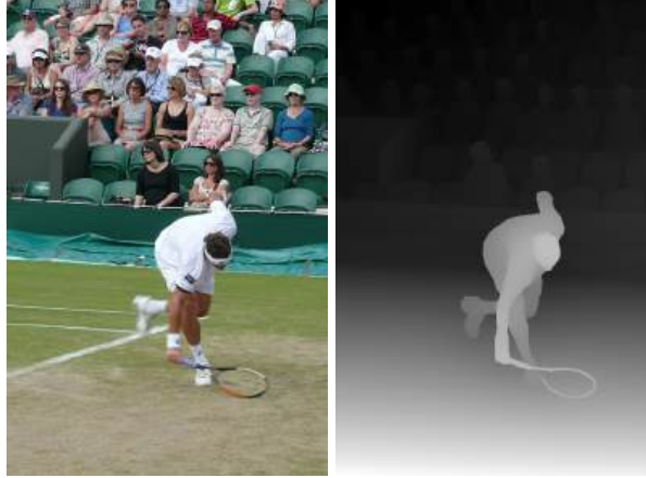
Figure 4.1: Example of a pseudo-label from the COCO dataset annotated by DepthAnythingV2. The left image shows the original COCO RGB image, and the right image shows the corresponding pseudo-label with relative inverse depth values.
