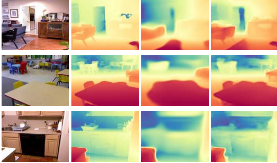
Figure 5.2: Qualitative results on the same ResNet50 model with and without skip connections between encoder and decoder. a) RGB input, b) ground truth depth map, c) without skip connections, d) with skip connections.
